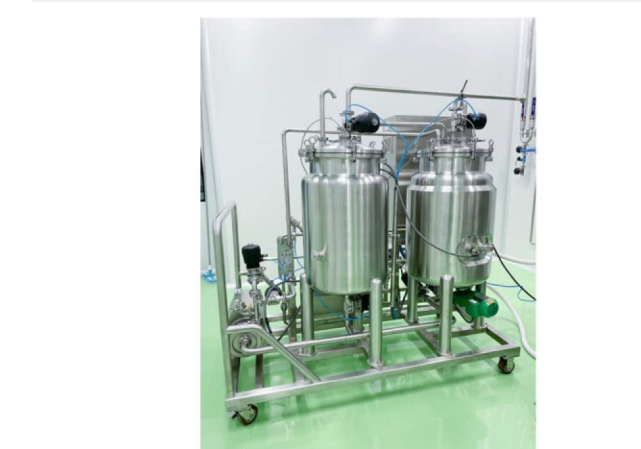
CIP 系统 CIP Process
