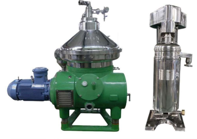
下游设备: 碟式离心机/管式离心机 Downstream Equipment: Disc Centrifuge/Tubular Centrifuge
